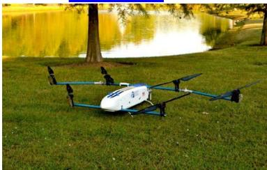
*This drone from Advanced Aircraft Company took first place in NIST's UAS Endurance Challenge with 112 minutes of flight time with a heavy payload.
