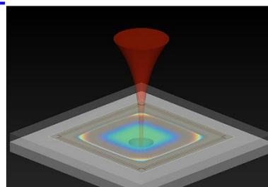
*Illustration of an optomechanical accelerometer, which uses light to measure acceleration.
