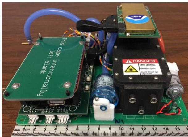
*NOAA CSL's Portable Optical Particle Spectrometer (POPS) uses an on-board laser to measure tiny suspended particles that influence stratospheric chemistry and reflect incoming sunlight. The miniaturized instrument, designed by CSL researchers in Boulder, Colorado, weighs 1.3 pounds and is about the size of a lunch box.
