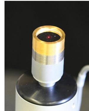
*Close-up of a microphone, with the laser spot hitting the center of its diaphragm.
